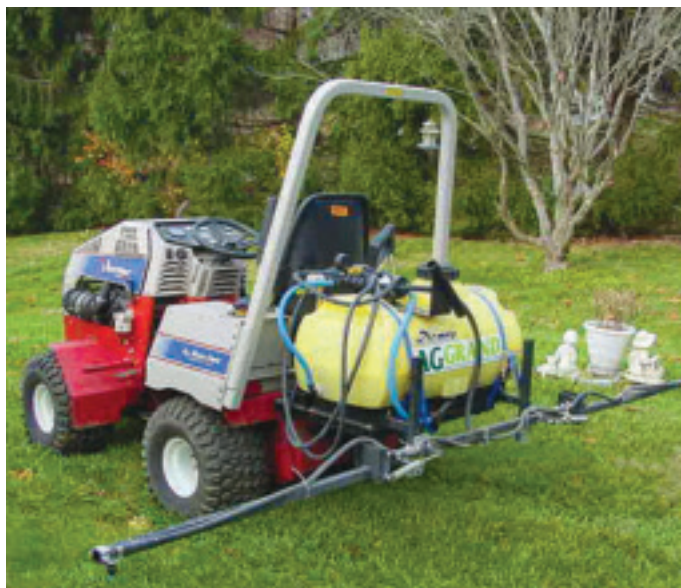
INNOVATIVE AGGRAND SPRAYER — Dealer Dave Richards Jr. of Maryland uses a 25-gallon tank with a Demco Sprayer to apply AGGRAND Natural Liquid Fertilizer. The sprayer is equipped with folding booms that allow Richards to spray 12 feet at a time. He uses #5 floodjet tips, driving at four miles per hour. It also has a hand gun with a 50-foot hose for trees and shrubs that spray 25 to 30 feet. He mixes one or two gallons of AGGRAND Liquid 4-3-3. Richards mixes one or two gallons of AGGRAND 4-3-3 Liquid Natural Fertilizer and AGGRAND Liquid Lime in the tank for per-acre application. The sprayer is mounted on the back of a 31 horse power Ventrac Diesel that has AMSOIL Synthetic Tractor Hydraulic/Transmission Fluid in the transmission and Series 3000 5W-30 Synthetic Heavy Duty Diesel Oil in the engine, with an EAO09 oil filter.
